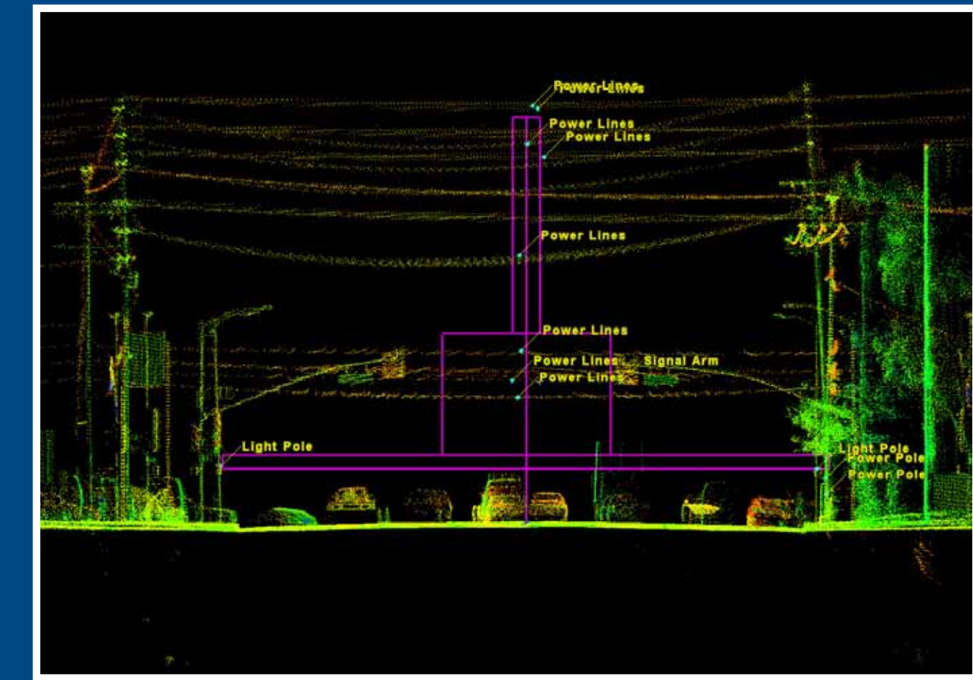
Vertical cross-section of innovative true scale cutting plane inserted into 3D point cloud
